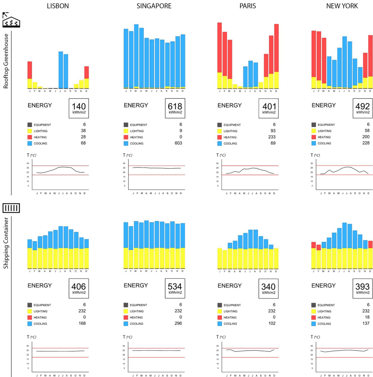
Figure 6: Energy loads (kWh/m 2 /y) and average indoor temperatures (°C) in the simulated urban farms.
