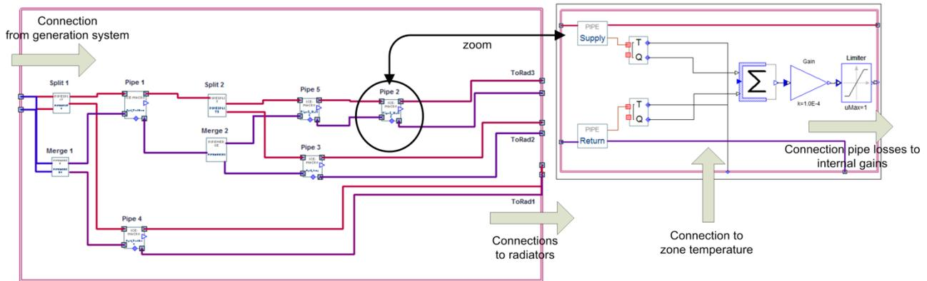
Figure 2. Example of IDA-ICE macro developed to model the simplified SH distribution system: a first layer combines a supply and a return pipe segment (right), the second layer (left) combines these two-pipe components into a network.
