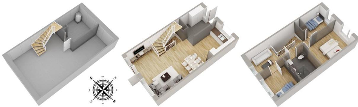
Figure 1. Floor plan of the terraced PH for the basement, ground and first floors, respectively.
