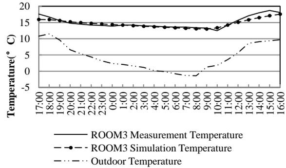
Figure 2: Comparison of field measurement and simulation
