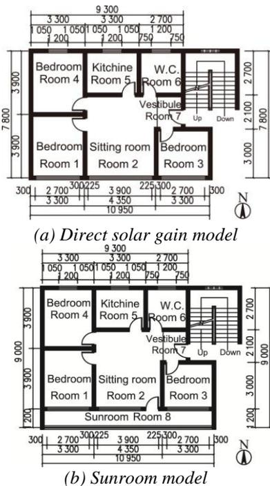
Figure 4: Layout drawings of basic models (Unit: mm)
