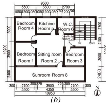
Figure 8: Schematic diagram of the sunroom depth models: a. depth 0.6 m; b. depth 2.4 m; (Unit: mm)
