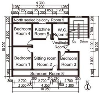
Figure 6: Layout drawing of double-balcony model (Unit: mm)
