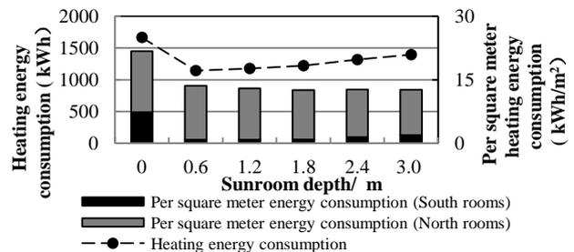
Figure 9: Simulation results of sunroom depth models
