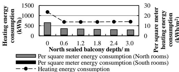
Figure 12: Simulation results of north balcony models
