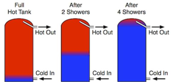
Figure 10: Schematic of the decentralised hot water storage tank operation principle. Four valves isolate the storage tank from the DHN. During the peak demand, the hot water from the tank is fully emptied. (Source: www.apricus.com)
