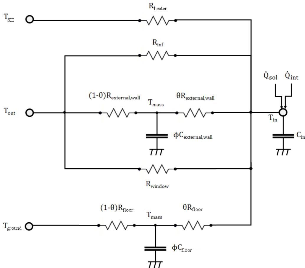
Figure 8: Schematic of the building model.  $T_{SH}$  is the water temperature inside the heater,  $\dot{Q}_{int}$  represents the internal gain, and  $\dot{Q}_{sol}$  represents the solar gains. External walls also represent losses through the roof.
