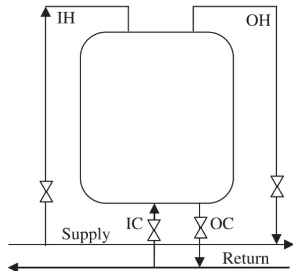
Figure 11: Schematic of the centralised storage tank. Four valves isolate the storage tank from the DHN. (Verda and Colella (2011))
