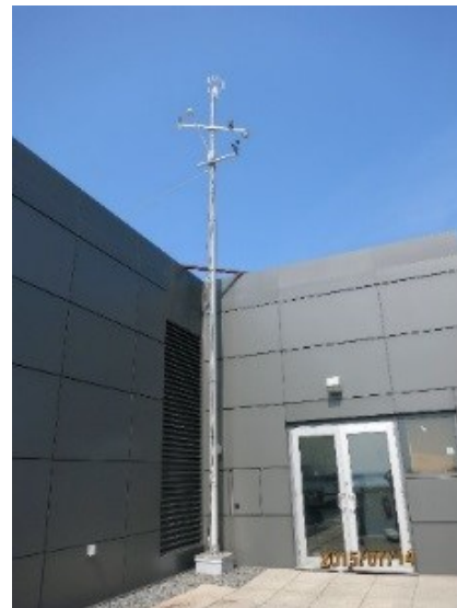
Figure 2: Weather station on the roof.
