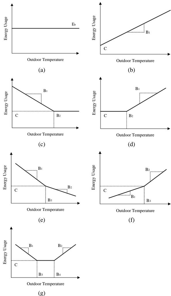
Figure 7: ASHRAE IMT Change-Point Models: (a) mean or 1P model; (b) 2P model; (c) 3P heating mode; (d) 3P cooling model; (e) 4P heating model; (f) 4P cooling model; and (g) 5P heating and cooling model.
