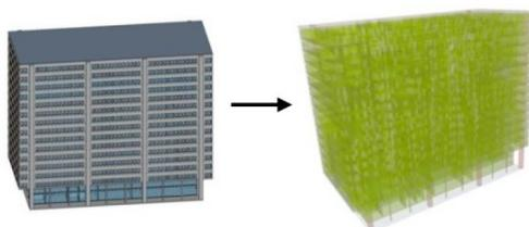
Figure 5. A GSA energy guidelines example: a BIM-based energy analysis starting with a BIM model exported to a model checker. Source: GSA (2016).
