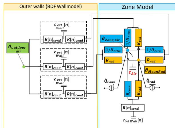
Figure 2: Network model of the IDA ICE 4.7 “CeSimZone”-model.
