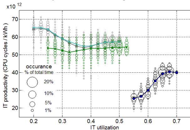
Figure 8 IT productivity versus DC utilization, mean part-load efficiency and performance spread
