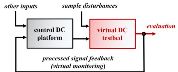
Figure 2 Schema of the virtual closed-loop testing
