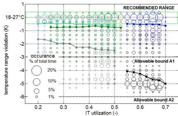
Figure 10 Temperature violation versus DC utilization, mean part-load efficiency and performance spread
