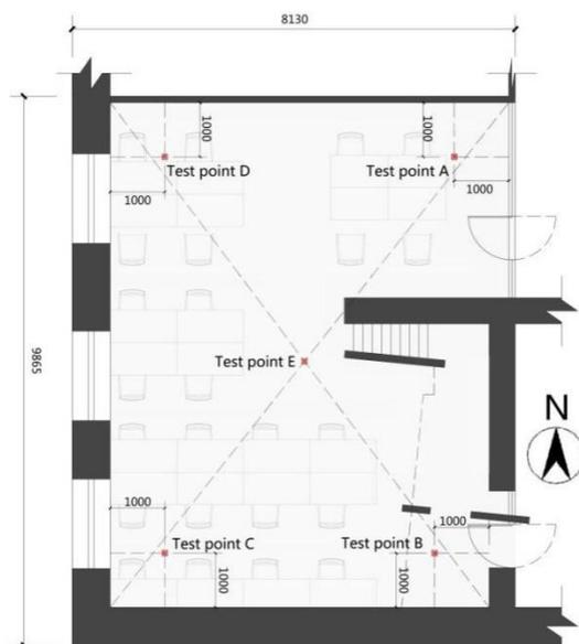
Figure 1: Layout of office staff and test points.
