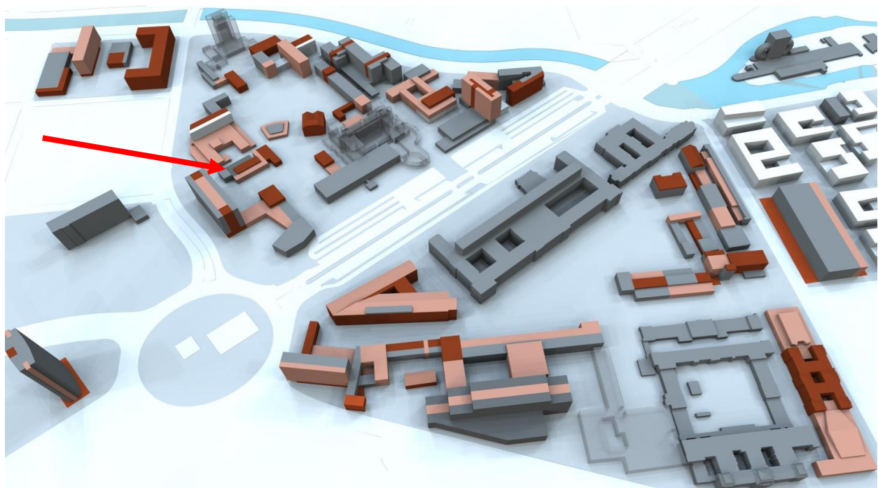
Figure 4: All thermal zones of 40 buildings on campus. The number of thermal zones varies between 2 and 9 for each building. The red arrow shows the example shown in figure 2.
