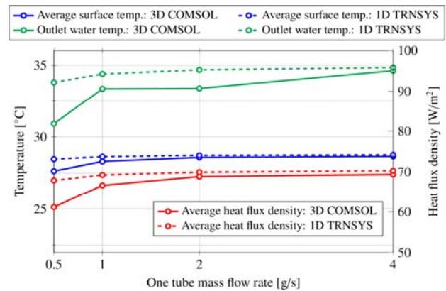
Figure 12: Steady state heating – U-shaped tubes
