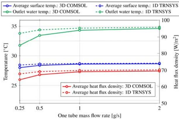
Figure 10: Steady state heating – straight tubes
