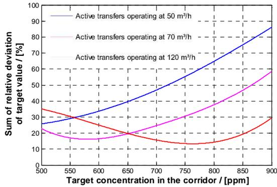
Figure 8: Sum of the relative deviation of the target values, for varying target CO<sub>2</sub> concentrations in the mixed air room (corridor).
