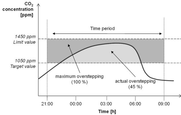
Figure 3: Illustration of the evaluation method for CO<sub>2</sub>-concentration.
