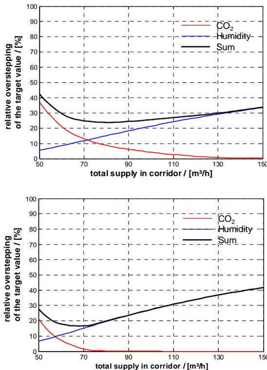
Figure 6: Relative deviation of the target values of carbon dioxide (1000 ppm) and humidity (30% relative humidity), as well as their sum in case of active transfers at 70 m<sup>3</sup>/h (above) and 150 m<sup>3</sup>/h (below) for varying global supply airflow rate in the corridor.
