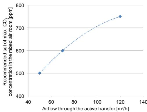
Figure 9: Planning guideline: recommended set point of max. CO<sub>2</sub> concentration in the mixed air room depending on the performance of the AOE.
