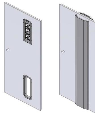
Figure 10: Sketch of the functional model of active transfer integrated directly into the door
