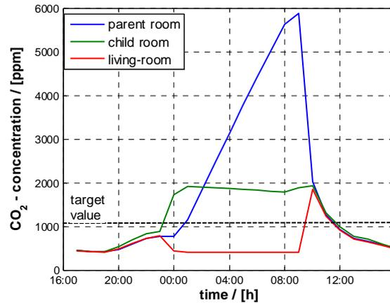
Figure 4: Simulation results of CO<sub>2</sub> concentration in parent bedrooms over night with no supply in the bedroom and no AOE between bedroom and mixed air zone.
