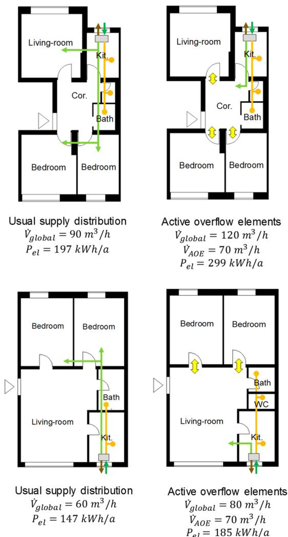
Figure 11: Results of the comparison between ventilation in cascade and with active transfers.
