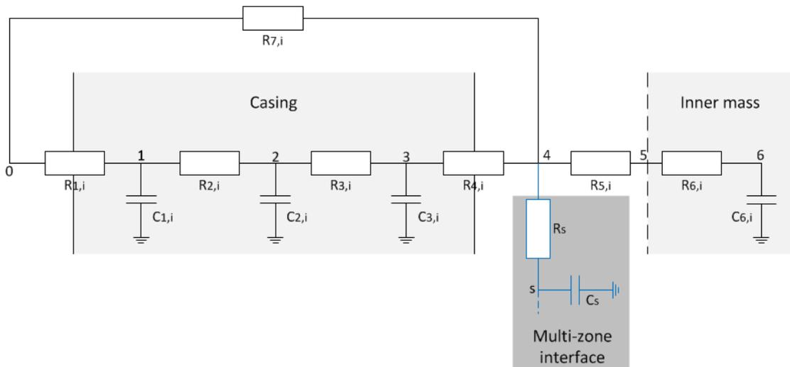
Figure 1 Thermal network of DIMOSIM mono-zone building model
