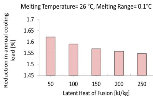
**Figure 7** Simulation trial-3 (latent heat varies) for Muscat
