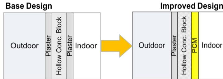
**Figure 4** Base wall design versus improved wall design
