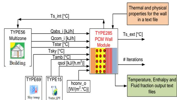
**Figure 1** Configuration of Type-285 within TRNSYS simulation studio
