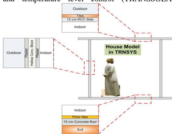
**Figure 2** Housing Model in TRNSYS simulation
