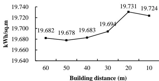
Figure 8 Relationship between building distance and energy consumption
