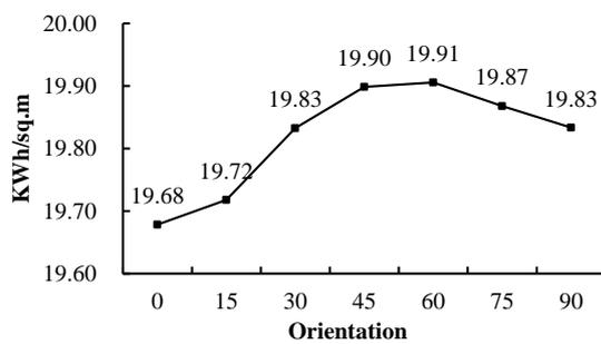
Figure 12 Relationship between energy consumption and orientation
