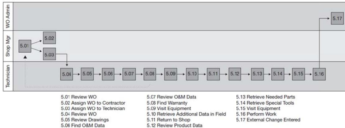
**FIGURE 6.12** Pre-COBie-enabled CMMS work order process collected by surveying three campuses.
