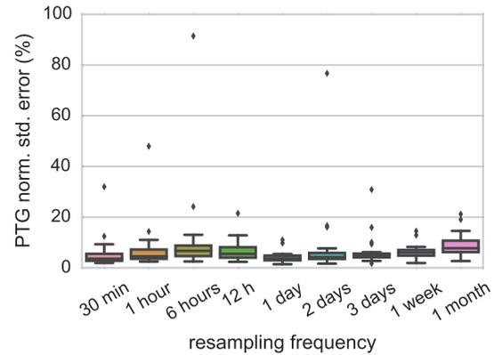
Figure 4: Power Temperature Gradient (PTG) standard error as a percentage of the parameter value for a range of resampling frequencies
