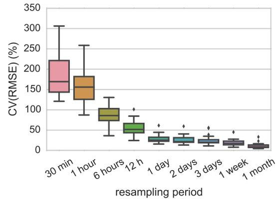
Figure 1: Plot of CVRMSE as a function of resampling frequency demonstrating rapid decrease in residual error with decreasing sampling frequency (longer averaging periods).
