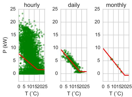
Figure 3: Power curves for site CTBLR01723 at hourly, daily, and monthly resampling frequencies.
