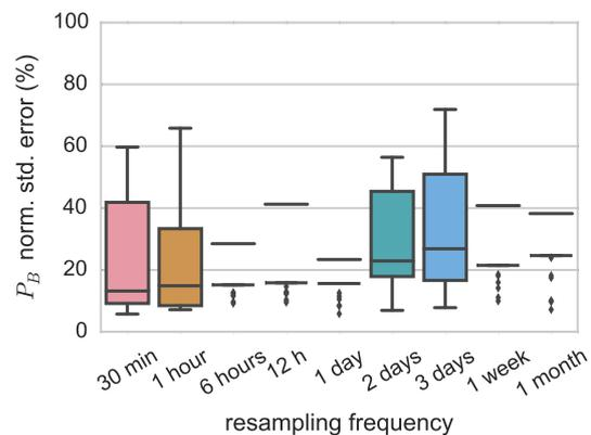
Figure 5: Baseload power ( $P_b$ ) standard errors as a percentage of parameter value for a range of resampling frequencies
