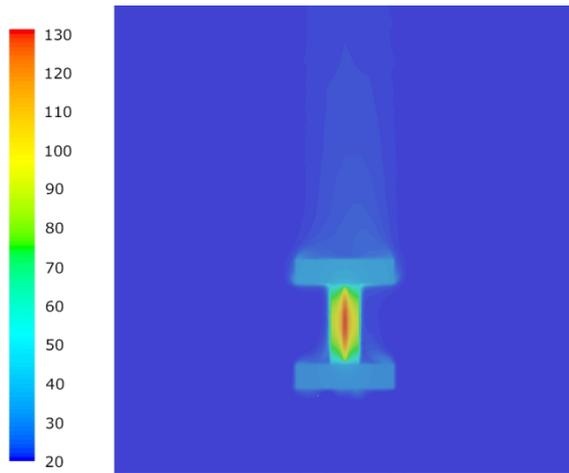
Figure 3: Simulated air temperature in the micro-climate (in °C, at  $P=43$  W, symmetry plane through the centre)
