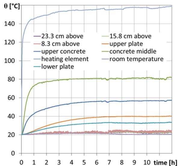
Figure 7: Heating until reaching steady-state ( $P=43 W$ )
