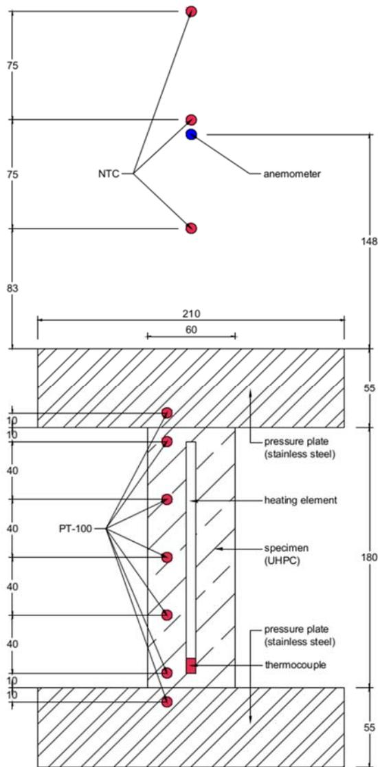
Figure 6: Vertical section of the measurement setup
