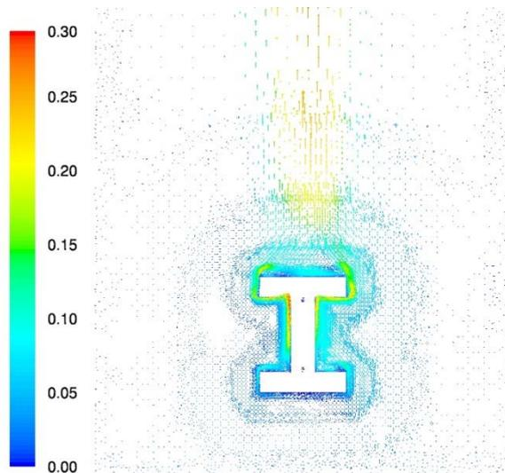
Figure 4: Simulated air velocity in the micro-climate (in m/s, at  $P=43$  W, symmetry plane through the centre)
