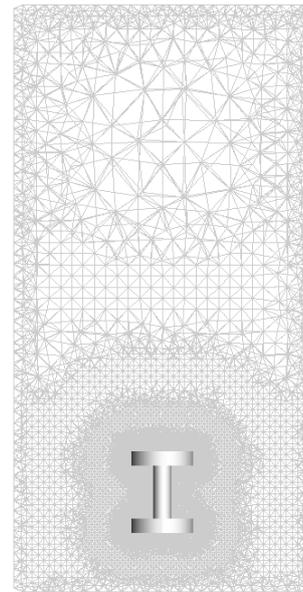
Figure 2: Mesh with local refinement surrounding the specimen
