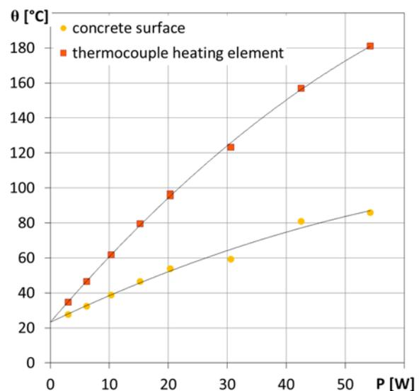
Figure 8: Temperature of the heating element (thermocouple) and concrete surface (middle PT-100) after reaching steady-state
