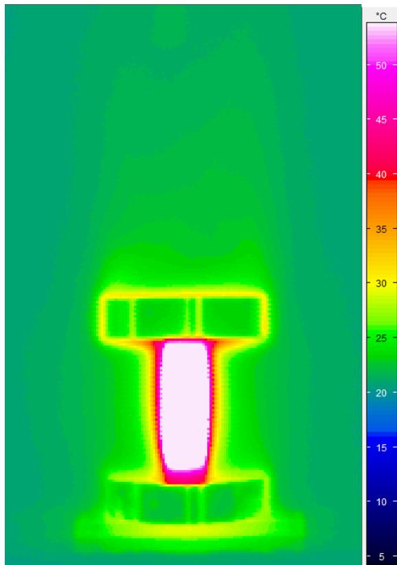
Figure 9: Thermography of the work plane ( $P=43W$ ), visualizing the temperature of the micro-climate
