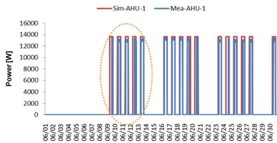
Figure 10 Comparison of measured and simulated AHU 1 fan power
