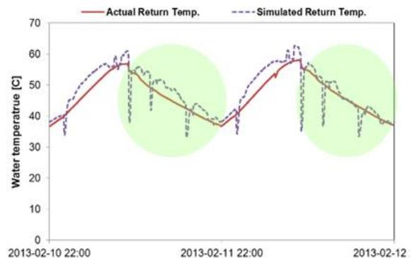
Figure 5 Comparison of measured and simulated boiler return water temperatures
