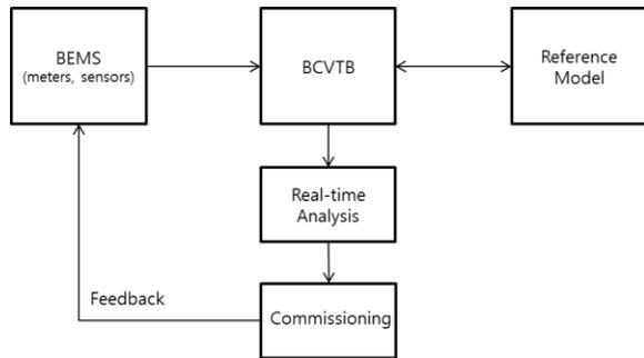
Figure 1 A framework of commissioning method using real-time energy performance
