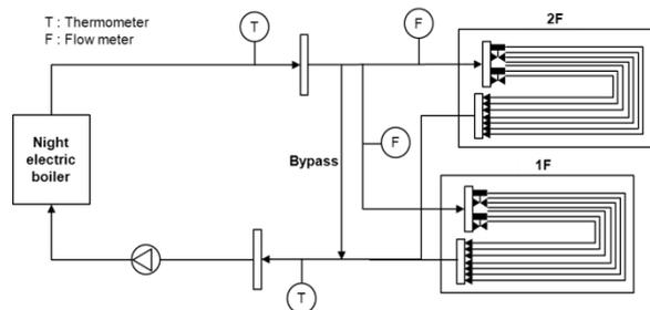
Figure 2 Schematic diagram of a radiant floor heating system with a night storage electric boiler in the 1st case building
