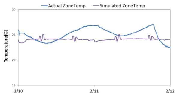
Figure 6 Comparison of measured and simulated zone temperature
