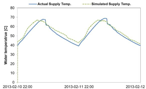
Figure 4 Comparison of measured and simulated boiler supply water temperatures
