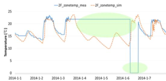
Figure 11 Comparison of measured and simulated 2F zone temperature
