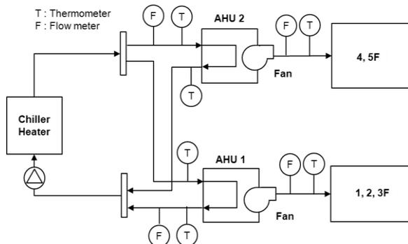
Figure 7 Schematic diagram of AHU systems with a chiller heater in the 2<sup>nd</sup> case building
