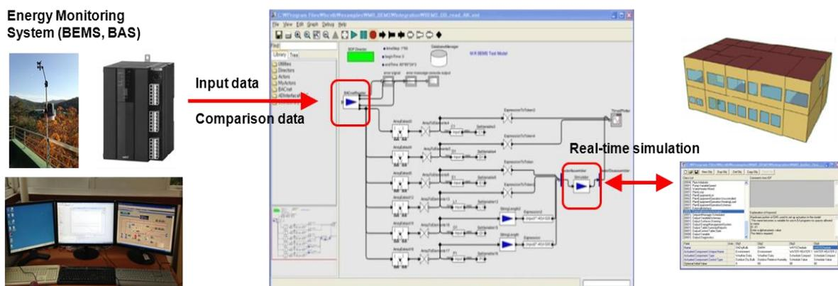
Figure 3 Real-time simulation system in the 1<sup>st</sup> case study
