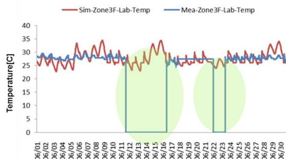
Figure 12 Comparison of measured and simulated 3F zone temperature
