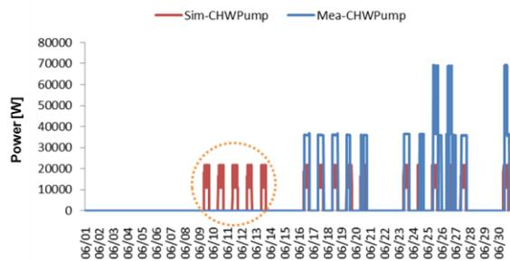
Figure 9 Comparison of measured and simulated CHW pump power
