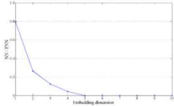
Figure 2 Embedding dimension using the FNN ratio
