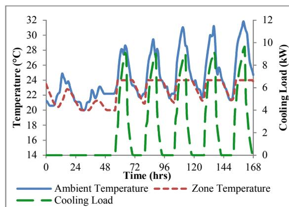
Figure 4 Reference building cooling load, ambient and zone temperatures for a week in July located in Atlanta, GA
