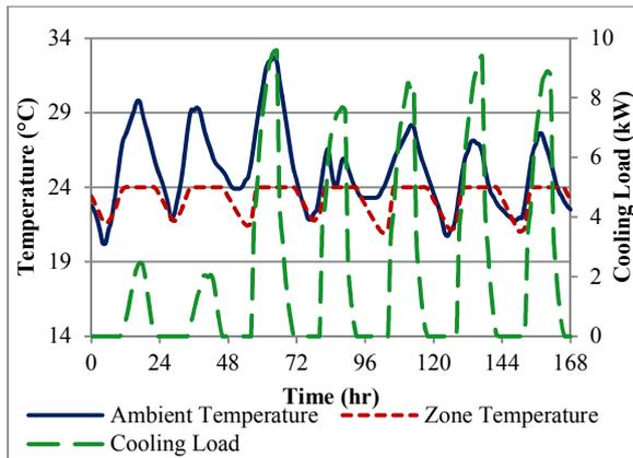
Figure 5 Reference building cooling load, ambient and zone temperatures for a week in July located in New York, NY
