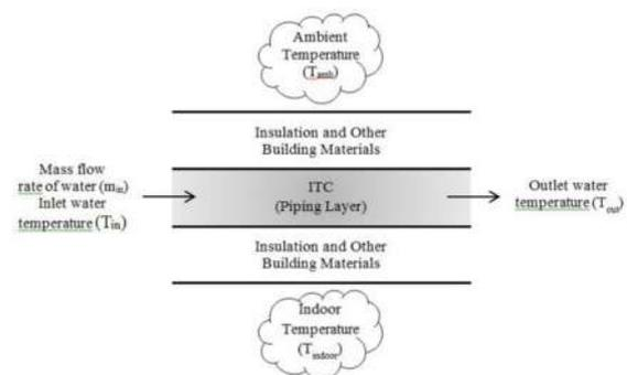
Figure 3 Schematic of ITC system in ceiling
