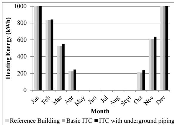
Figure 10 Heating energy comparison for buildings simulated in Atlanta, GA
