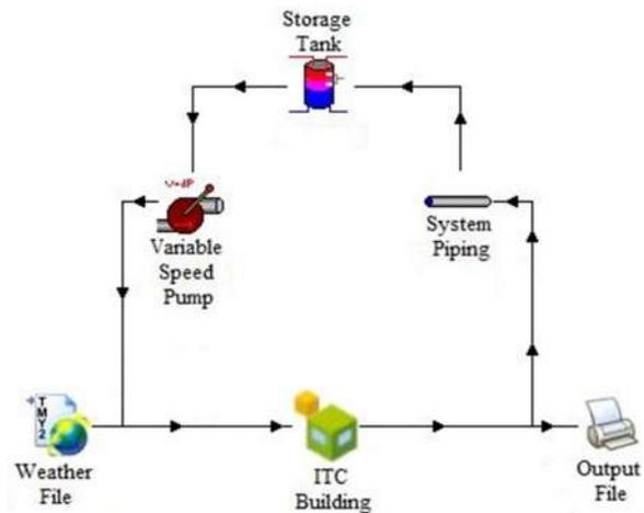
Figure 2 Dynamic model of TRNSYS with ITC either perfectly insulated or buried underground
