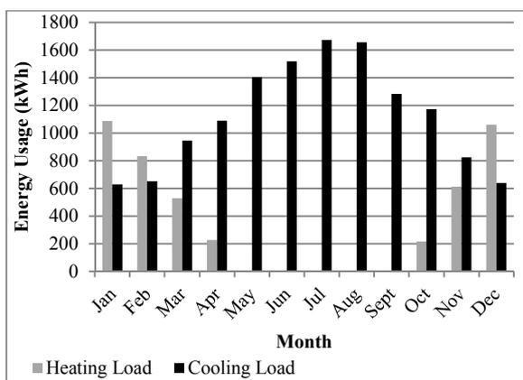
Figure 6 Reference building's monthly heating and cooling energy required in Atlanta, GA
