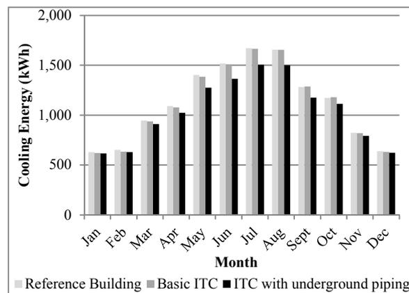
Figure 8 Cooling energy comparison for buildings simulated in Atlanta, GA
