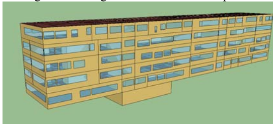
Figure 1 Geometry of the Energy Model in OpenStudio Plugin for SketchUp
