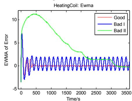
Figure 7 EWMA of Error Index for Heating Coil
