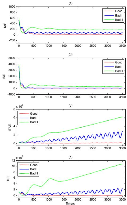
Figure 9 Integral Based Index for Cooling Coil
