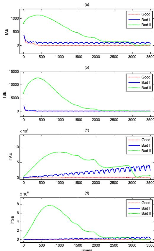
Figure 6 Integral Based Index for Heating Coil Control
