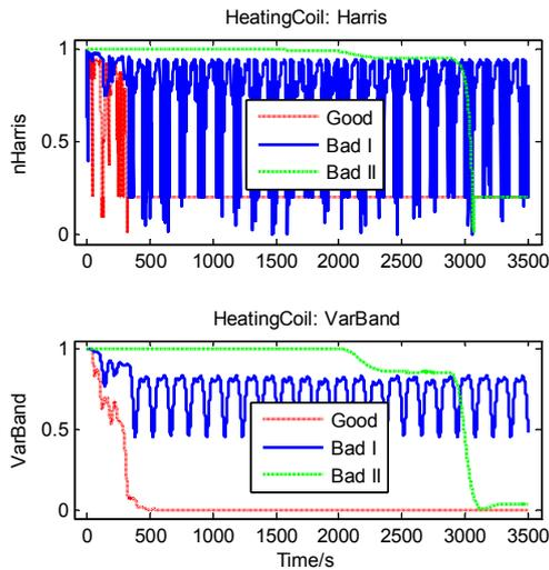
Figure 8 Variance Based Index for Heating Coil
