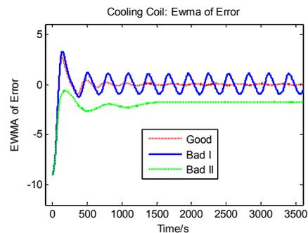
Figure 10 EWMA of Error Index for Cooling Coil
