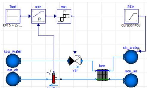
Figure 3 Diagram of Modelica Models for Cooling Coil Model in Dymola
