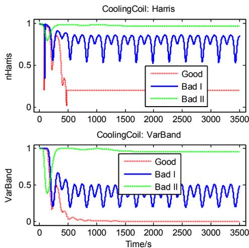
Figure 11 Variance Based Index for Cooling Coil
