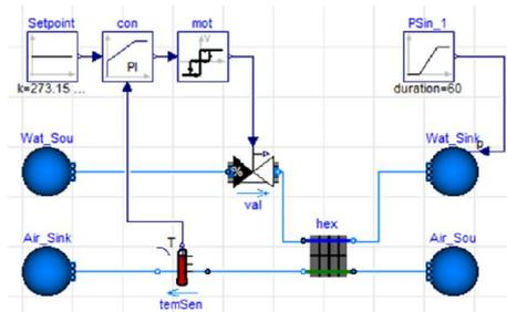
Figure 1 Diagram of Modelica Models for Heating Coil Model in Dymola
