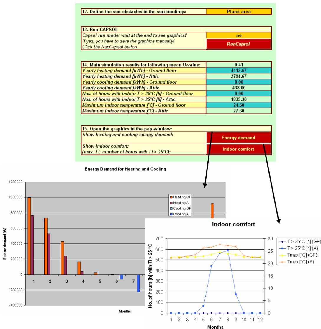
Fig. 3 Excel VBA based interface of the generic model for the assessment of the heating and cooling energy demand of detached houses - final table with selected result types and two buttons displaying either energy demand or thermal comfort chart (the abbreviation "GF" means Ground Floor and "A" stands for Attics)
