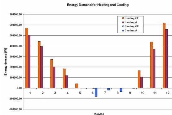
Fig. 9 Energy demand chart for lightweight house – shaded location (mean  $U$ -value =  $0.31 \text{ W}/(\text{m}^2.\text{K})$ )
