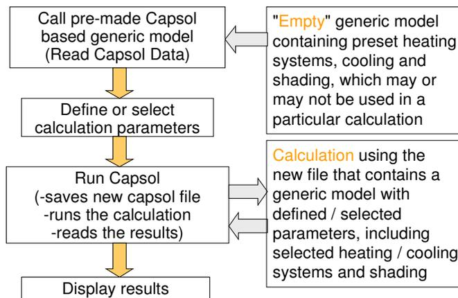
Fig. 2 Simplified working scheme of the Excel VBA based interface
