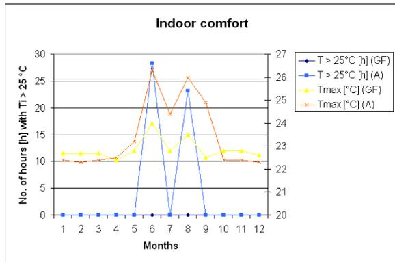
Fig. 5 Indoor comfort chart for brick-based (heavy) house having mean  $U$ -value =  $0.31 \text{ W}/(\text{m}^2.\text{K})$  and situated in the forrest / city (shaded location) – secondary y-axis indicates monthly mean max.  $T$
