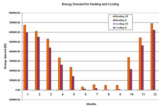
Fig. 8 Energy demand chart for heavy brick-based house – shaded location (mean  $U$ -value =  $0.31 \text{ W}/(\text{m}^2.\text{K})$ )
