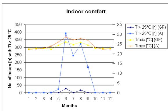
Fig. 7 Indoor comfort chart for wood-frame house (lightweight) having mean  $U$ -value =  $0.31 \text{ W}/(\text{m}^2.\text{K})$  and situated in the forrest / city (shaded location) – secondary y-axis indicates monthly mean max.  $T$
