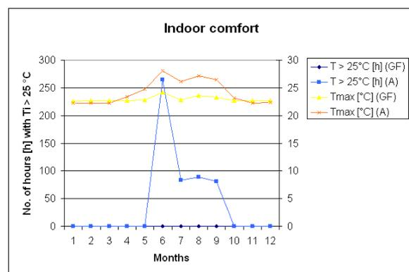
Fig. 4 Indoor comfort chart for brick-based (heavy) house having mean *U*-value = 0.41 W/(m<sup>2</sup>.K) and situated on the plane (unshaded location) – secondary y-axis indicates monthly mean max. *T*
