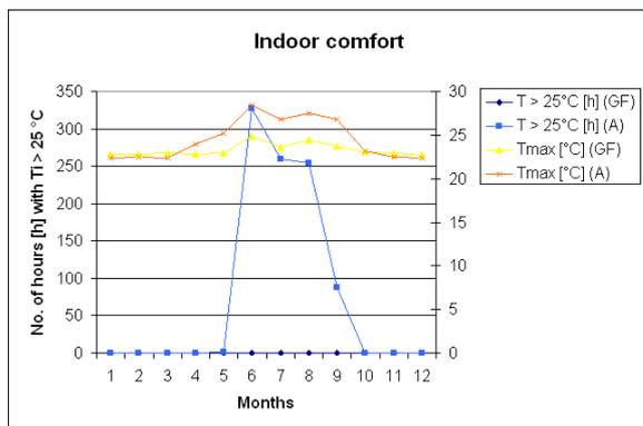
Fig. 6 Indoor comfort chart for wood-frame house (lightweight) having mean  $U$ -value =  $0.41 \text{ W}/(\text{m}^2.\text{K})$  and situated on the plane (unshaded location) – secondary y-axis indicates monthly mean max.  $T$
