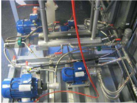
Figure 3 Water pump and electrolyte recirculation.
