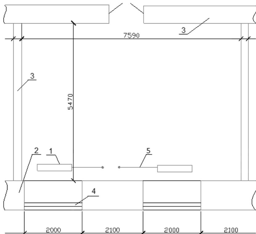
Figure 1 A schematic illustration of simulation object (a) plan of a room, (b) axonometric scheme of the one-pipe heating system: 1 - heating appliance; 2, 3 – interior and exterior envelopes; 4 – multiple glass pane; 5 - water pipe
