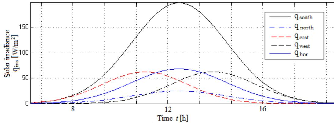
Figure 3 Daily solar irradiance  $q_{ins}$  ( $W/m^2$ ) toward the surface of the different spatial orientation (Tomsk, January):  $q_{south}$  – vertical south orientation surface,  $q_{north}$  – vertical north orientation surface,  $q_{east}$  – vertical east orientation surface,  $q_{west}$  – vertical west orientation surface,  $q_{hor}$  – horizontal surface
