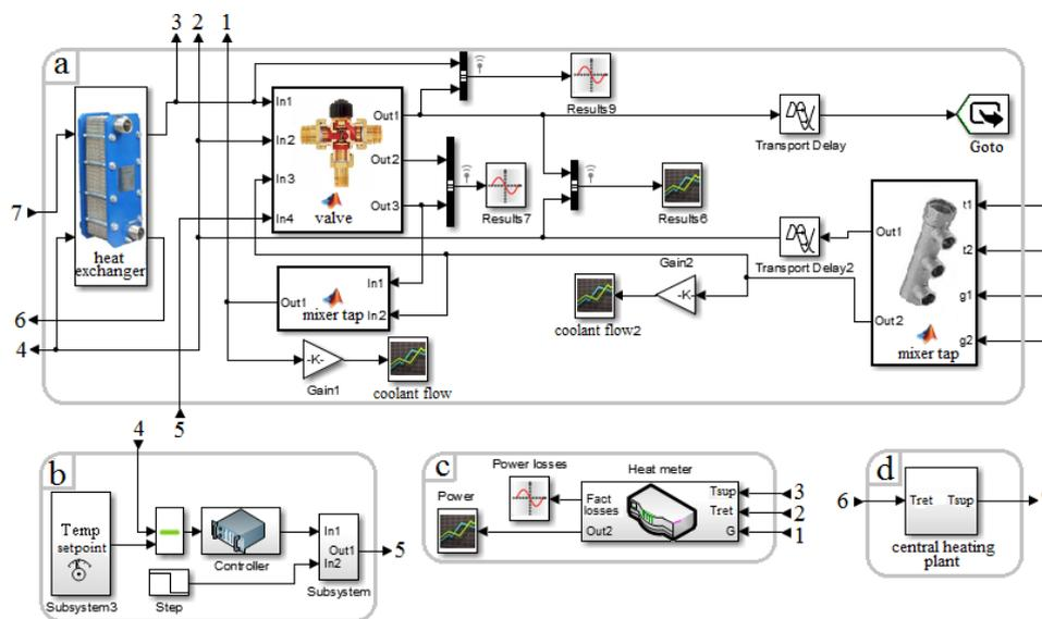
Figure 2 The main blocks of the thermal model of the heating system: (a) blocks of individual heating plant; (b) controller of heat consumption; (c) heat calculator; (d) heat supply source
