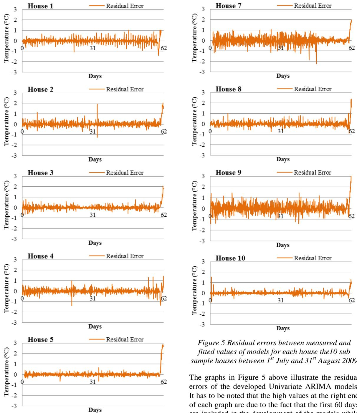
Figure 5 Residual errors between measured and fitted values of models for each house the 10 sub sample houses between 1<sup>st</sup> July and 31<sup>st</sup> August 2009
