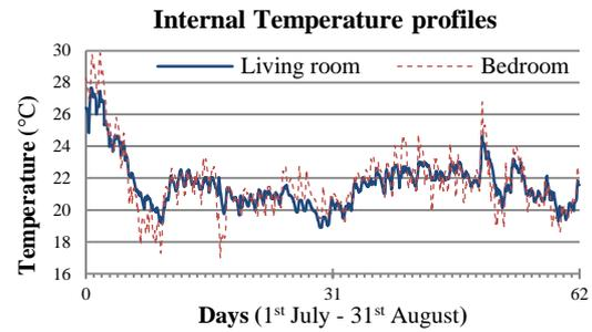
Figure 1 Hourly measured room air temperatures of example home between 1<sup>st</sup> July and 31<sup>st</sup> August 2009
