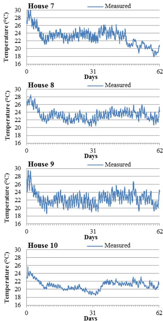
Figure 4 Hourly room air temperatures measured in living rooms of 10 sub sample houses between 1<sup>st</sup> July and 31<sup>st</sup> August 2009
