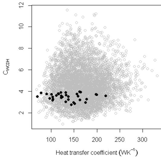
Figure 7:  $C_{WCDH}$  against the total heat transfer coefficient. The 33 optimal buildings in terms of minimizing  $C_{WCDH}$  and  $C_{PMVH}$  are shown by dark circles
