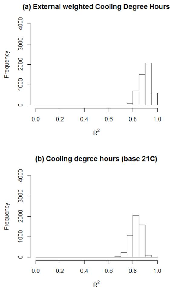
Figure 3: Histogram of the  $r^2$  values for linear regression for internal WCDH against (a) external WCDH and (b) CDH (base temperature of 21 °C).
