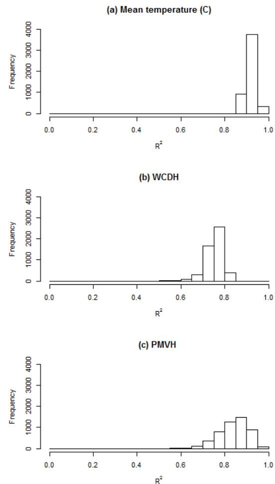
Figure 2: Histogram of the  $r^2$  values for linear regression for (a) internal mean summer temperature, (b) internal WCDH and (c) internal PMVH against the external mean summer temperature
