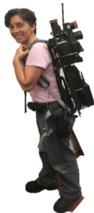
Figure 1 Generation 3 RAPMOD and operator
