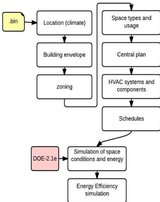
Figure 3 General workflow for energy simulation in EE4
