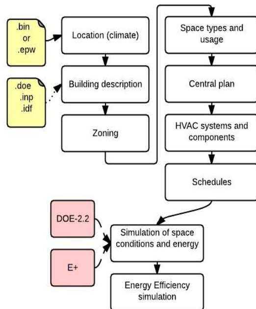
Figure 5 General workflow for energy simulation in SIMEB
