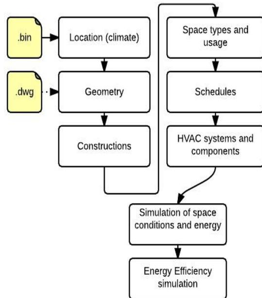
Figure 7 General workflow for energy simulation in eQUEST
