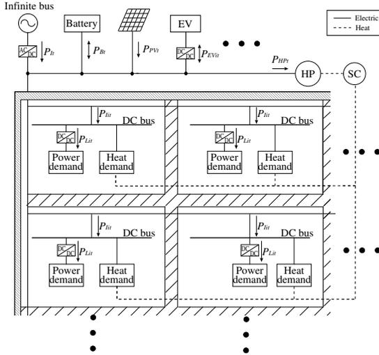
Figure 1 The smart apartment model
