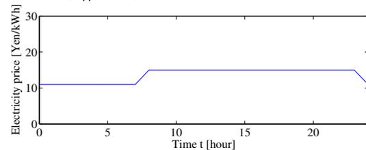
Figure 8 Electricity price for high voltage receiving.
