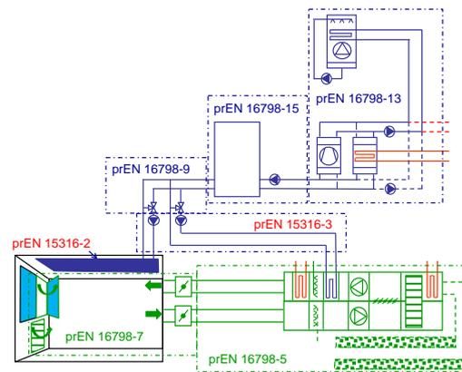
Figure 2 System schematic with the covered areas of the different standards
