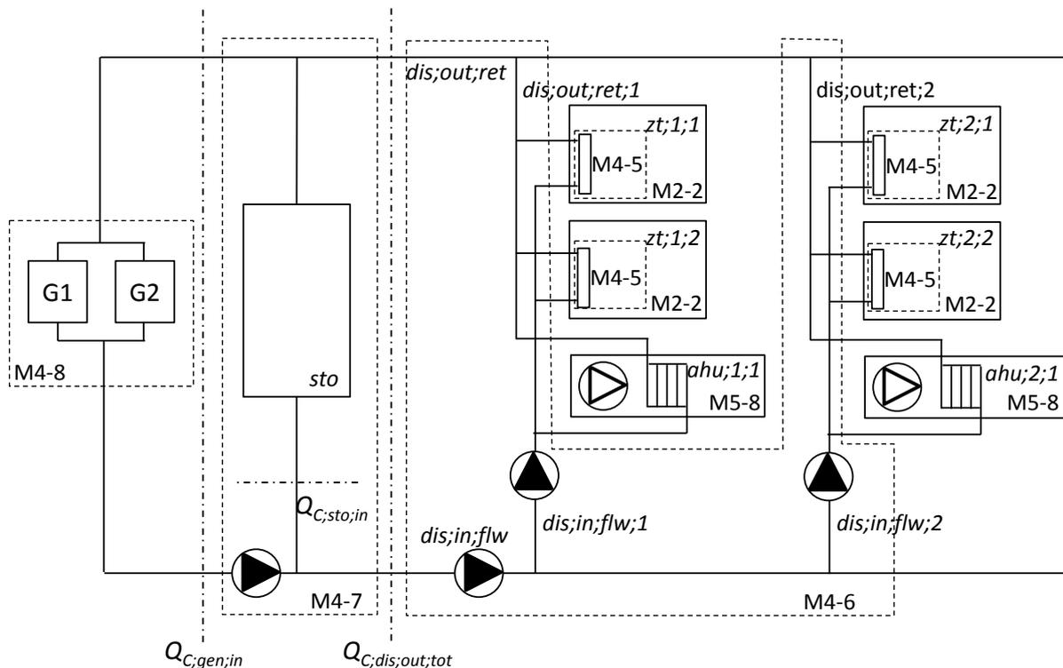
Figure 4 Cooling system scheme with module boundaries and nomenclature given in prEN 16798-9
