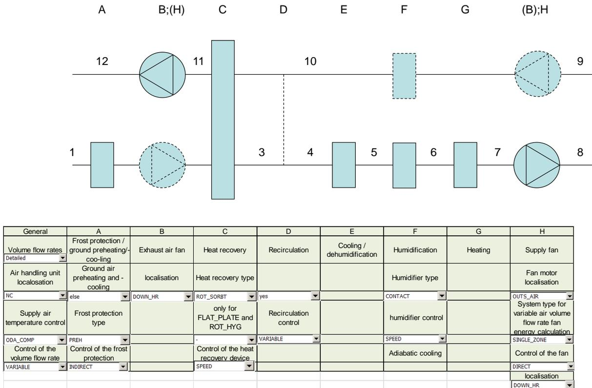
Figure 3 Ventilation/AC-system scheme and technology choice options in prEN 16798-5-1
