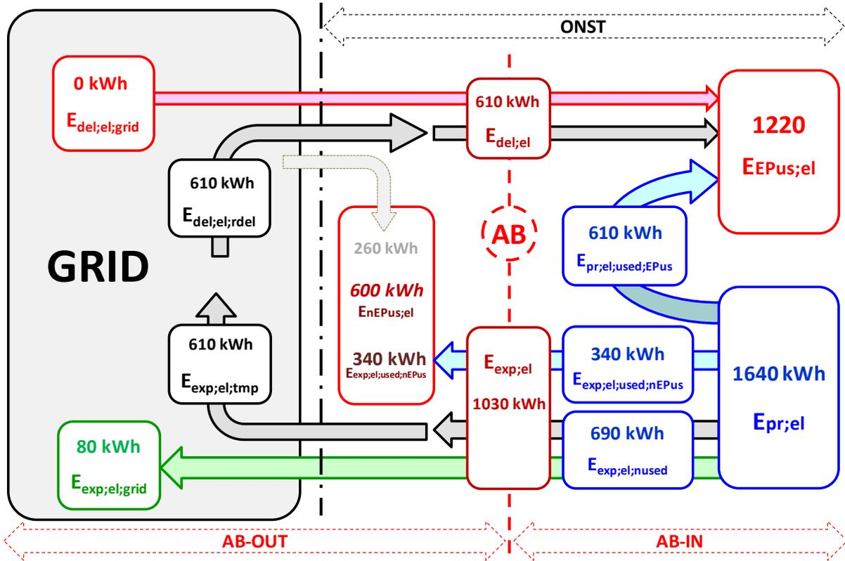
Figure 1 Reference diagram for the energy balance of electric energy in the OAS
