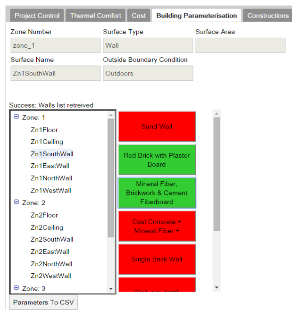
Figure 7: An example of the Expert System while performing parametric settings on different wall constructions.
