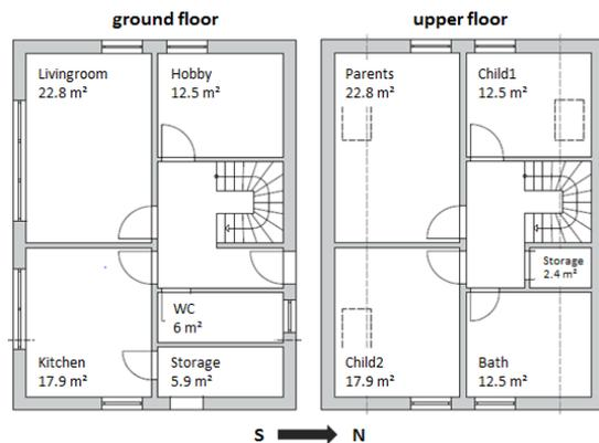
Figure 1: Floor plan of the typical one-family dwelling in AixLib
