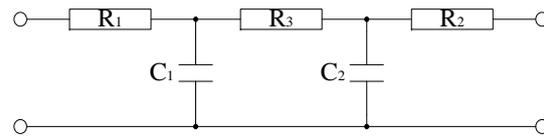
Figure 2: Resistance-capacitance concept for a multi-layer wall model
