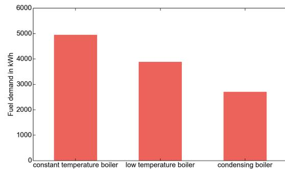
Figure 6: Simulated fuel demand for one apartment with different boiler types
