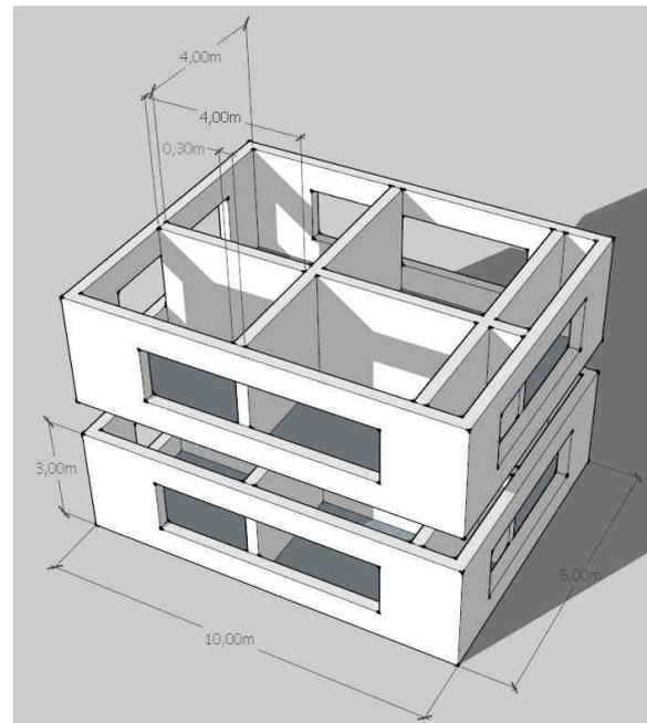
Figure 2 Geometry model for the parameterisation of the low-order building model in the case of the single family house
