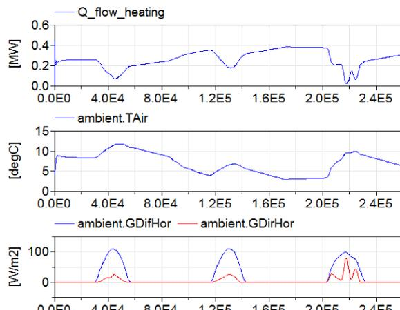
Figure 8 Overall heating load of all buildings of the street village and used climate data (outside temperature, horizontal irradiation)
