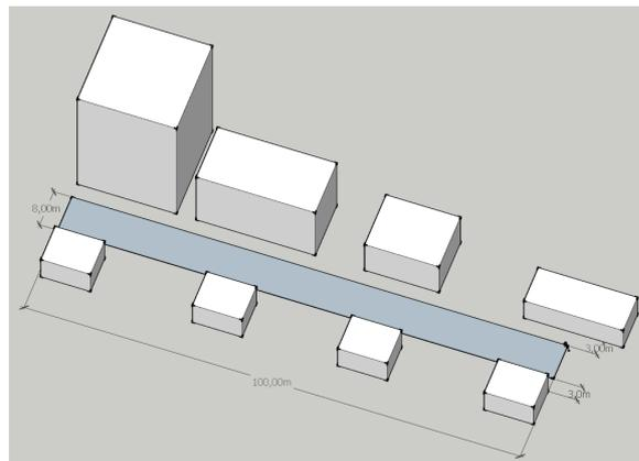
Figure 3 Street model (length = 100 m, width = 8 m, distance to buildings = 3 m) width 8 uniformly distributed building models: 4 SFH, 1 SDH, 1 SMFH, 1 MMFH, 1 LMFH
