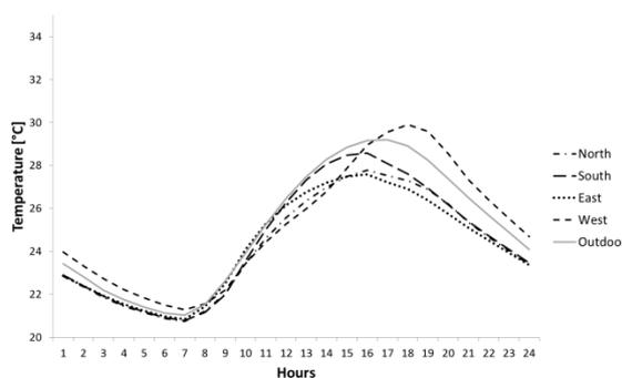
Figure 10: Simulated indoor temperatures for a typical summer day (July-September) of rooms oriented differently (northern wing, first floor) excluding the effect of sun protections (scenario BSNS)
