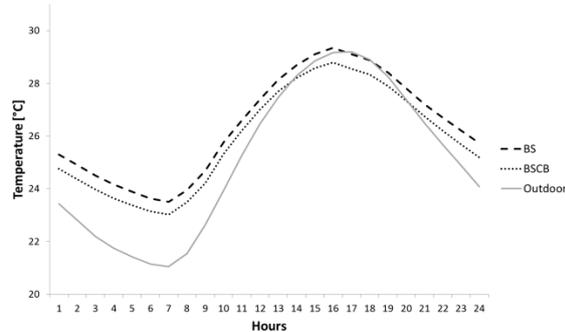
Figure 14: Simulated indoor temperatures for a typical summer day (July-September) of eastern rooms, the second floor of the northern wing (scenarios BS and BSCB)
