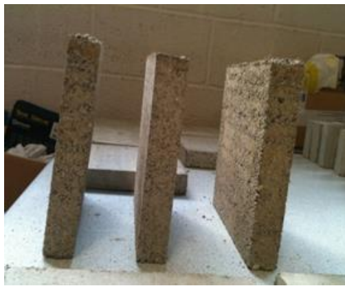
Figure 4: L75 Samples used for the measurement of thermal conductivity.
