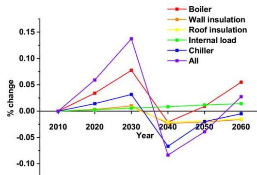
Figure 2. Evolution of the total energy consumption of the building for different ageing parameters by decade.
