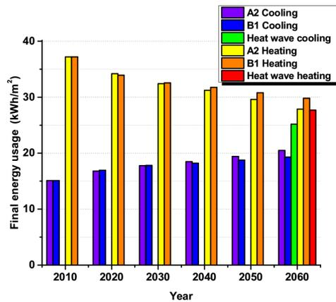
Figure 1. Cooling and heating final energy usage for the Torino building for scenarios A2, B1 and the heat wave. Simulations were run from present (2010) to 2060 in decadal steps.
