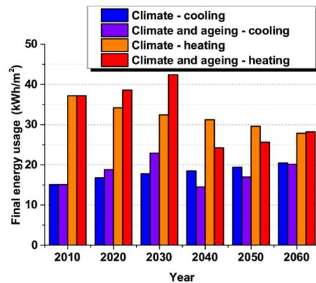
Figure 4. Final heating and cooling building energy usage under climate scenario A2 for the cases of climate change without ageing and climate change plus ageing. The building is retrofitted in year 2040.
