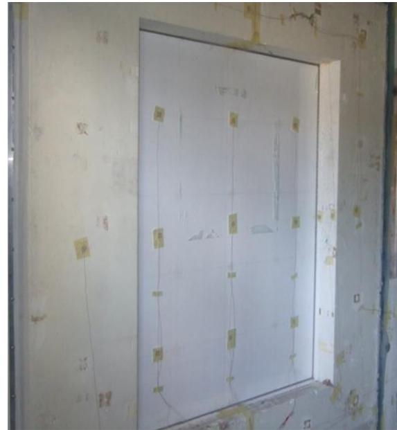
Figure 7 One of calibration panels mounted into the surround panel – warm side view
