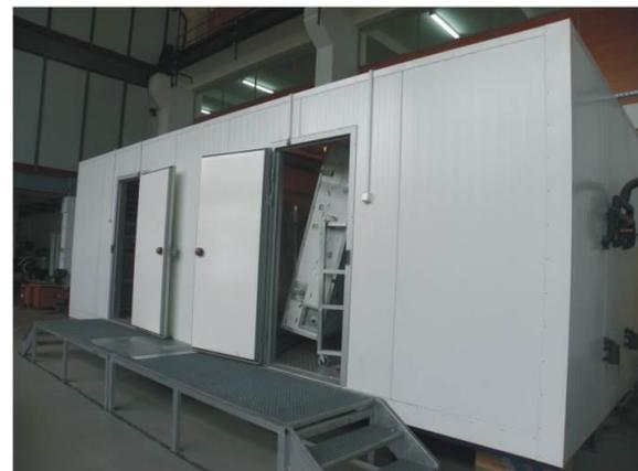
Figure 6 General view of calorimetric hot box (CHB) system
