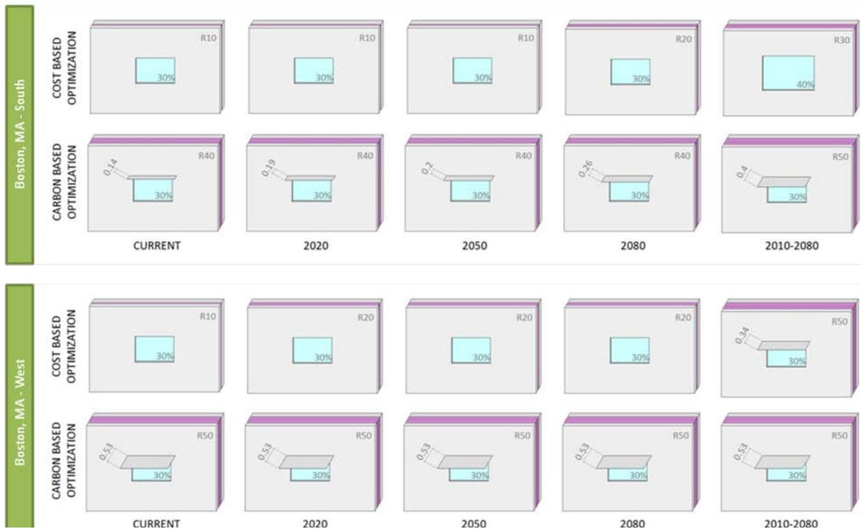
Figure 2 - Sample of optimized results from study, the south and west facades in Boston, MA.
