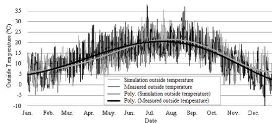
**Figure 9.** Comparison between outside temperature measured and given by simulation software (Poly = polynomial interpolation)
