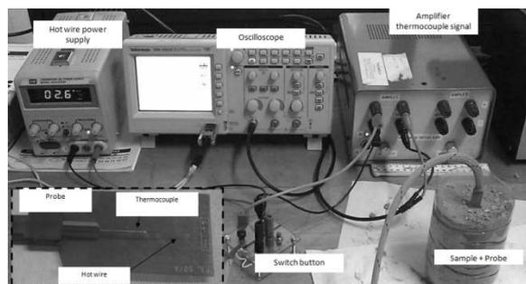
Figure 6 : Hot wire method - Assembly procedure
