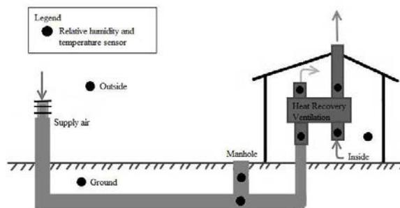
Figure 2. Deployment of relative humidity and temperature sensors
