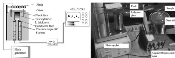
Figure 5 : Flash method - Assembly procedure
