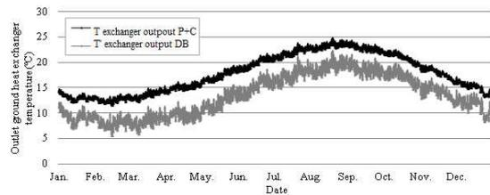
**Figure 7.** Comparison between exchanger output temperature in P+C and DB software
