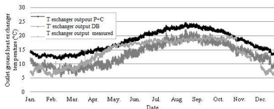
**Figure 10.** Comparison between measured exchanger output temperature and exchanger output temperature from P+C and DB software (simulation weather file)
