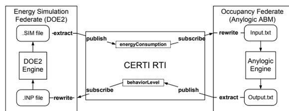
Figure 1: Data flow of energy simulation federation (adapted from Menassa et al. 2013)
