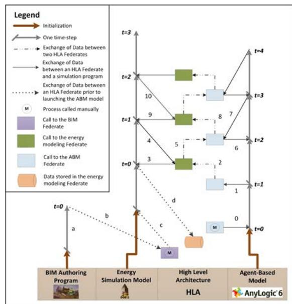
Figure 3: Data Synchronization and Function Call through HLA (Refer to Steps a-d and Steps 0-10 for detailed description of the different interactions)
