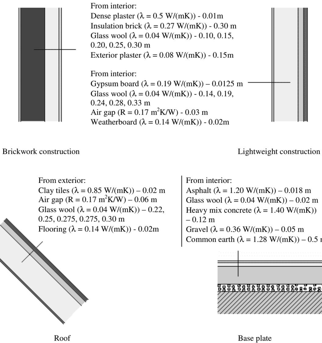
Figure 5 Composition of the main parts of the building envelope as modeled using Capsol's Wall Type Editor
