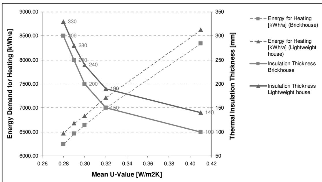
Figure 7 The effect of the mean U-value [W/(m<sup>2</sup>.K)] improvement on the annual reduction of energy demand for heating [kWh/a] in dependence upon thermal insulation thickness [mm] (indicated on the secondary y-axis)
