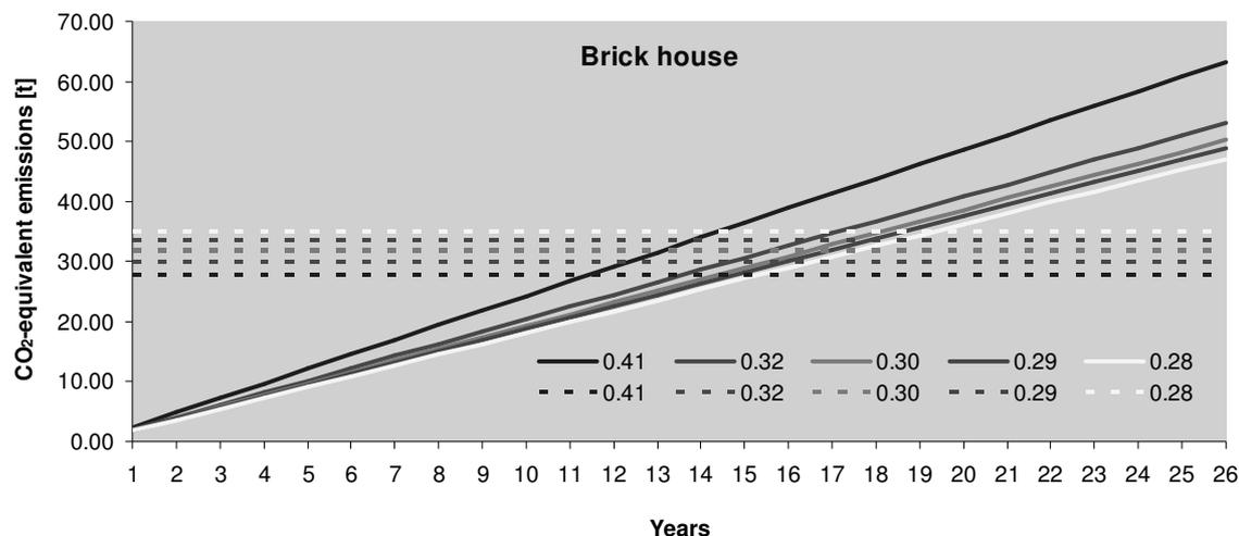
Figure 8 Relationship between the embodied equivalent CO<sub>2</sub> (GWP) emissions (dotted lines) and CO<sub>2</sub> emissions due to the operation (continuous lines) of the demonstration brick house for five mean U-values of the building envelope
