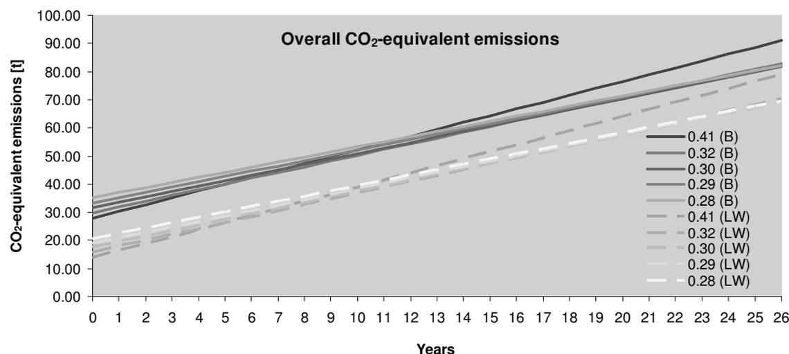
Figure 9 Course of overall CO<sub>2</sub>-equivalent emissions for investigated demonstration objects – brick house (B) and lightweight house (LW)
