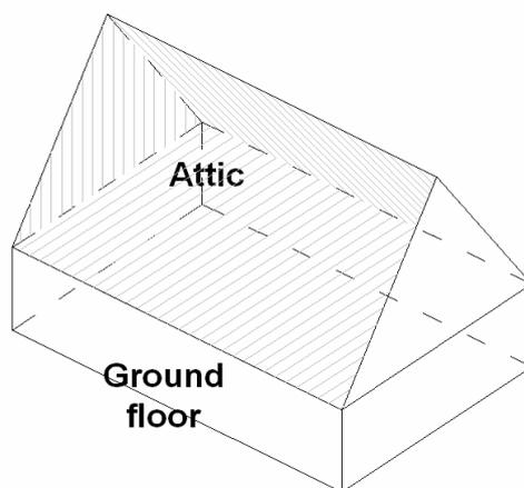
Figure 6 Division of the model in two thermal zones
