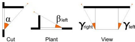
Figure 5 – Definition of the angles of sun protection
