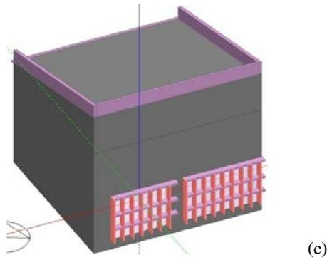
Figure 4(a,b,c) – Model with brises-soleil, created in Design Builder software. Southeast facade
