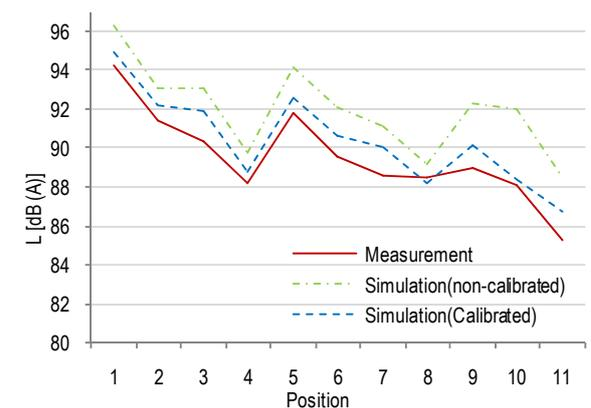
Figure 12 Measured and simulated (non-calibrated and calibrated) pre-retrofit sound distribution in OP
