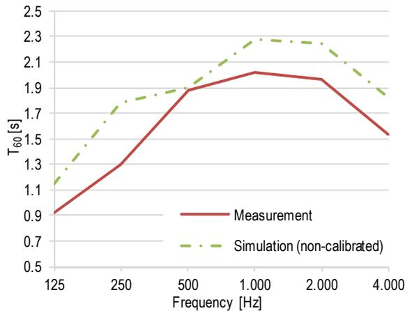
Figure 7 Measured and simulated (non-calibrated) reverberation times in SR (non-occupied)
