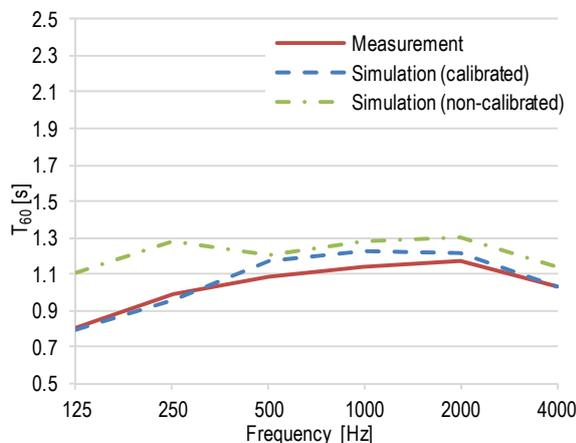
Figure 9 Measured and simulated (non-calibrated and calibrated) post-retrofit reverberation times in SR (non-occupied)
