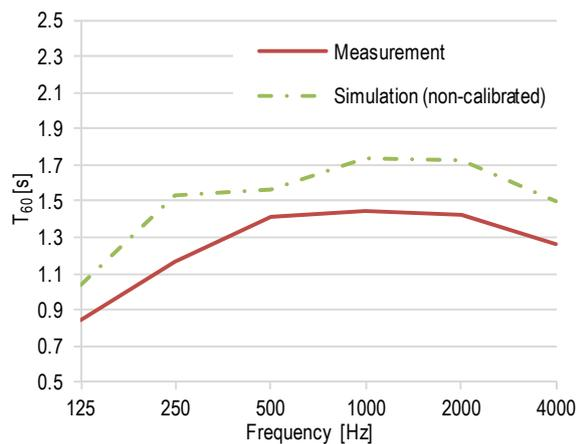
Figure 8 Measured and simulated (non-calibrated) reverberation times in OP (non-occupied)
