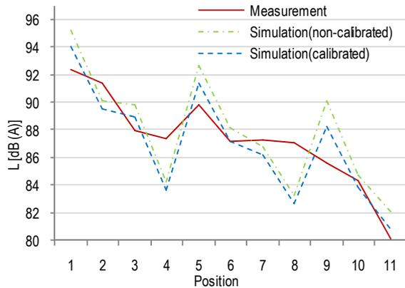
Figure 13 Measured and simulated (non-calibrated and calibrated) post-retrofit-sound distribution in OP
