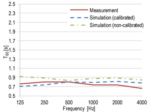
Figure 10 Measured and simulated (non-calibrated and calibrated) post-retrofit reverberation times in OP (non-occupied)
