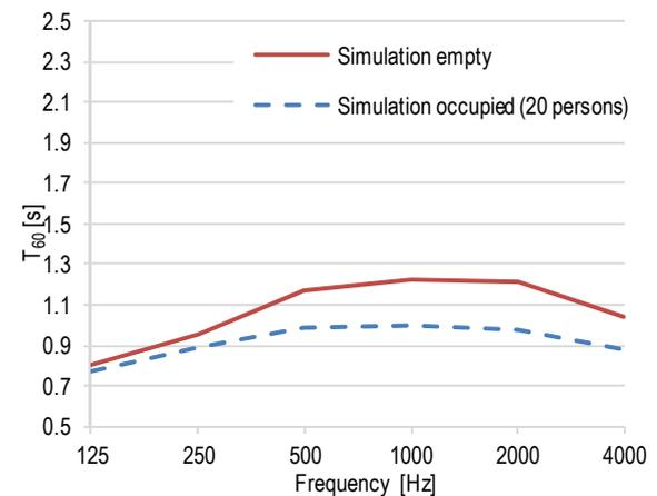
Figure 11 Simulated (calibrated) post-retrofit reverberation times in SR under non-occupied and occupied (20 people) conditions
