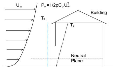
Figure 1 Pressure difference at the opening
