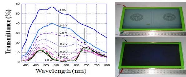
Fig. 1 The UW designed ECW of 12 inch × 20 inch, (left) transmission change and (right) photos of the ECW at transparent (above) and colored stage (below) (Xu et al., 2004; Kim et al., 2009).
