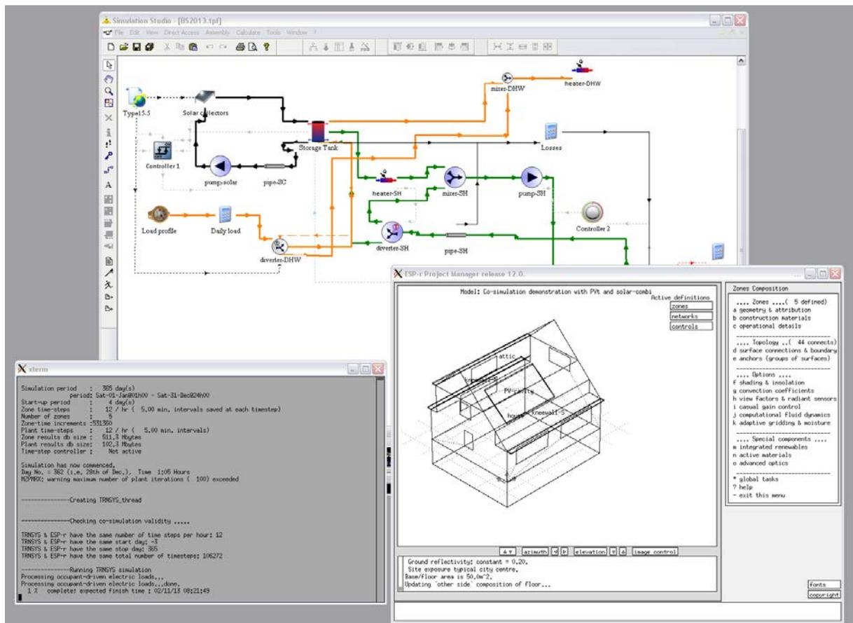
Figure 2: Co-simulation session: model inputs created through TRNSYS (top) and ESP-r (bottom right) interfaces with a co-simulation running in a Cygwin xterm (bottom left)
