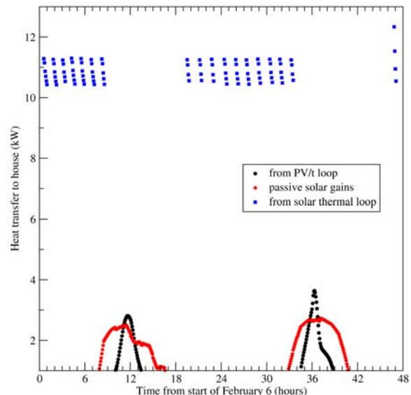
Figure 6: Solar thermal, PV/t, and passive solar input to house over two days in February
