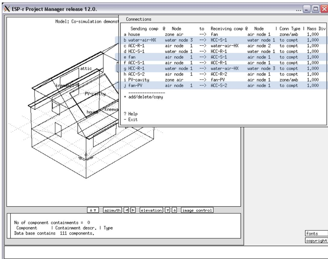
Figure 5: ESP-r plant network connections including couplings to TRNSYS
