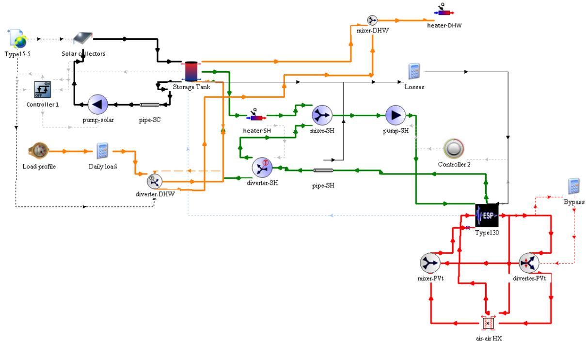
Figure 4: TRNSYS network including Type 130 for coupling to ESP-r
