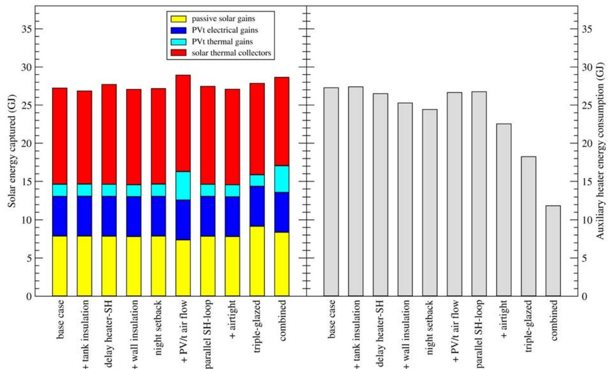
Figure 8: Impact of individual measures on solar energy gains and auxiliary heating consumption integrated over heating season
