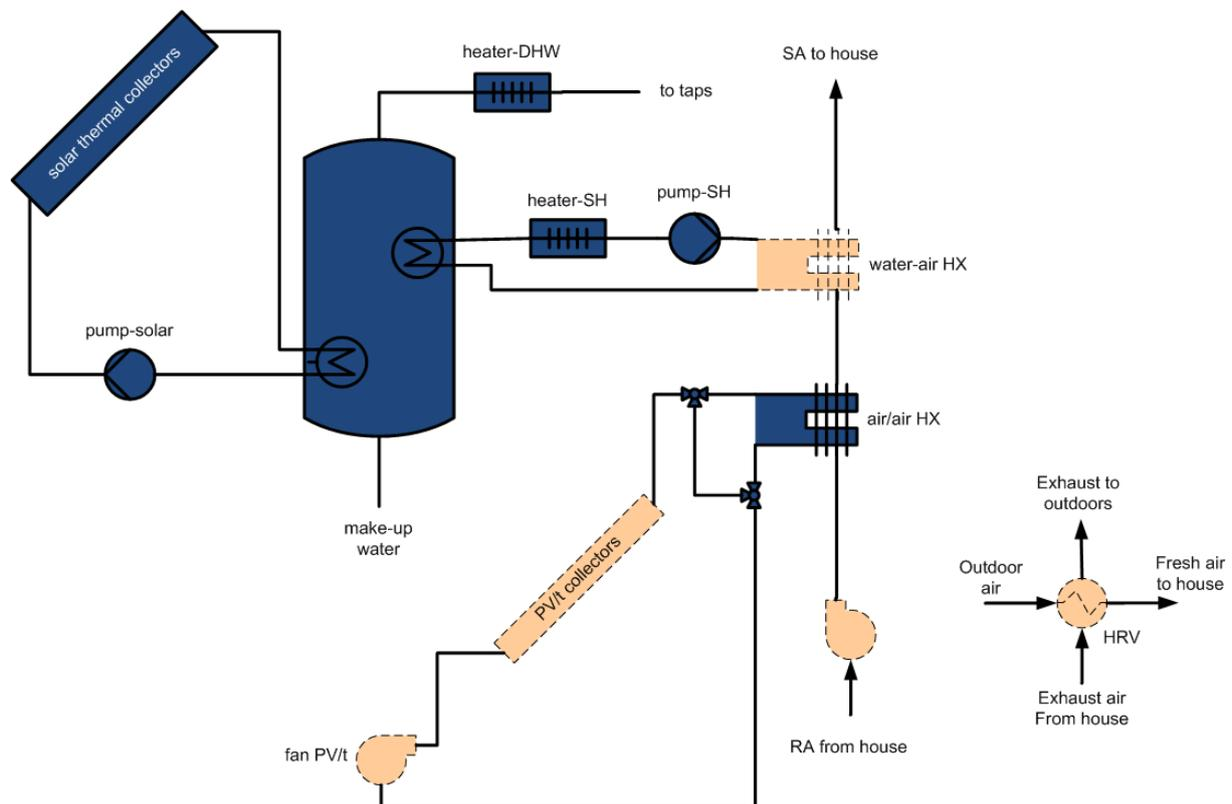
Figure 3: Collaborative simulation of solar and mechanical systems by ESP-r (components shown in light orange) and TRNSYS (components shown in dark blue)
