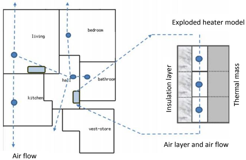
Figure 4: Simulation models for a one-bedroom flat with Quantum space heaters
