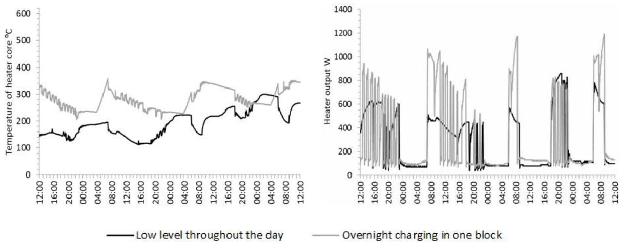
Figure 6: Impact of alternative charging schedule on storage utilisation and on heat output
