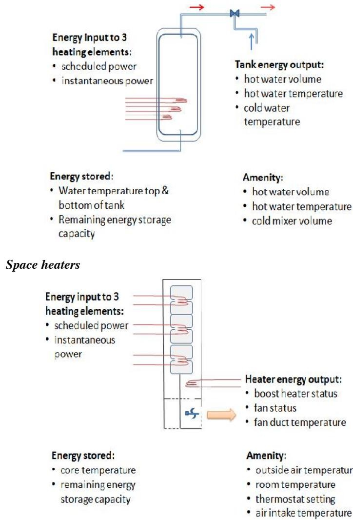
Figure 2: The DDSM monitoring scheme
