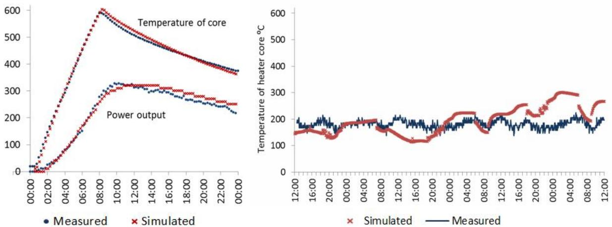
Figure 5: Calibration of heater models: a) laboratory test data for uncontrolled output and b) field measurements
