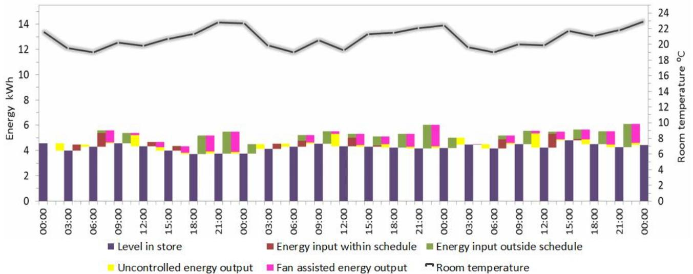
Figure 3: 3-hourly energy balances in a storage heater over 3 successive days
